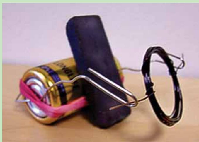
*Explanation:* Electrical energy from the cell 'flows' through the paper clips to the coil and back to the cell, making the coil an electromagnet. This electromagnet is repelled by the bar magnet which starts the coil turning. The remaining enamel switches the coil electromagnet off and the coil turns until it is switched on again. This is repeated and keeps the motor turning.
