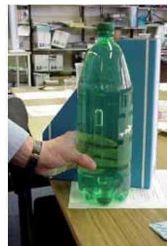
*Explanation:* When you increase the pressure on the bottle, the air bubble in the glass tube is forced into a smaller volume so the tube sinks. When the pressure is removed, the air expands and the diver returns to the top.
